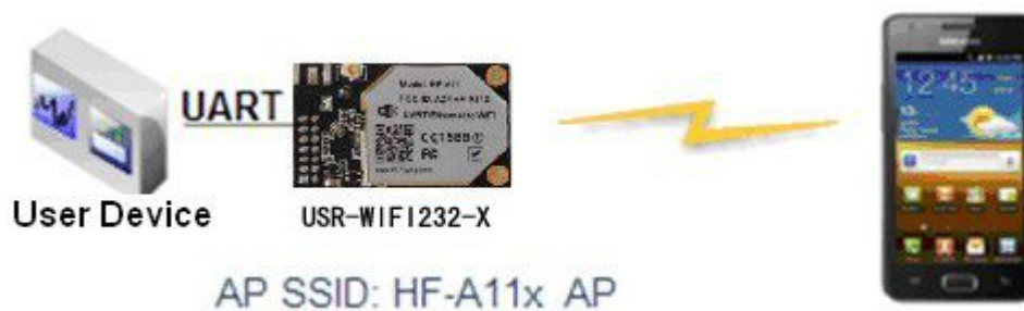
Figure 34 Wireless Control Application
