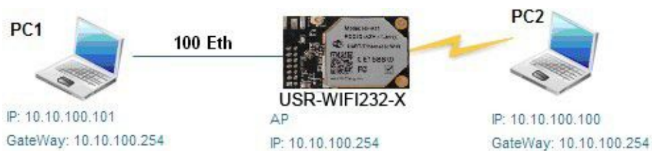
Figure 19 USR-WIFI232-X Ethernet Interface Networking (As AP)
