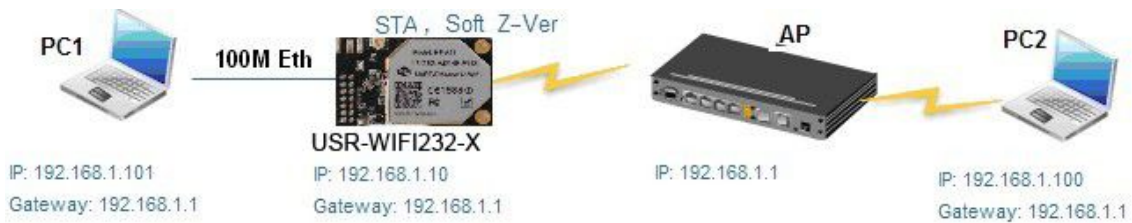
Figure 21 USR-WIFI232-X Ethernet Interface Networking (As STA, Z-Ver)
