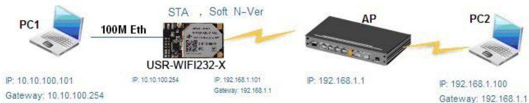
Figure 20 USR-WIFI232-X Ethernet Interface Networking (As STA, N-Ver)
