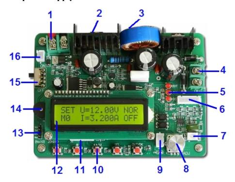
1.DC input 2.Power MOS transistors 3.Filter inductance 4.DC output
